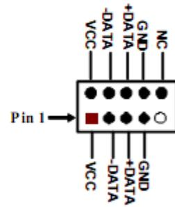
(9) COM2/4/6/5 (9-Pin): Serial Port Header
